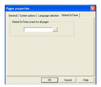
Global on timer allows you to specify the name of a global procedure to be periodically and independently executed on the active page. Such a procedure may be effectively used to constantly test one or more PLC variables and to emit alarm messages, for example through asynchronous messages (see 4.3.4).
